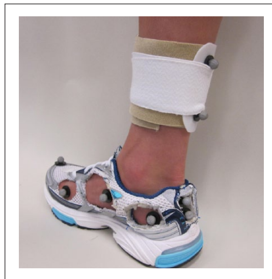
Figure 4. Marker set-up for kinematic data collection.
